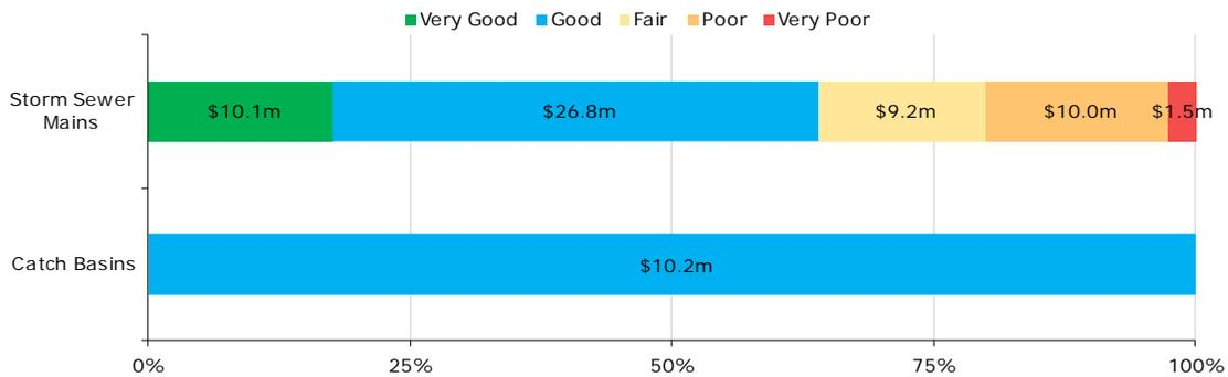
To ensure that the Township’s Storm Network continues to provide an acceptable level of service, the Township should monitor the average condition of all assets. If the average condition declines, staff should re-evaluate their lifecycle management strategy to determine what combination of maintenance, rehabilitation and replacement activities is required to increase the overall condition of the Storm Network.
