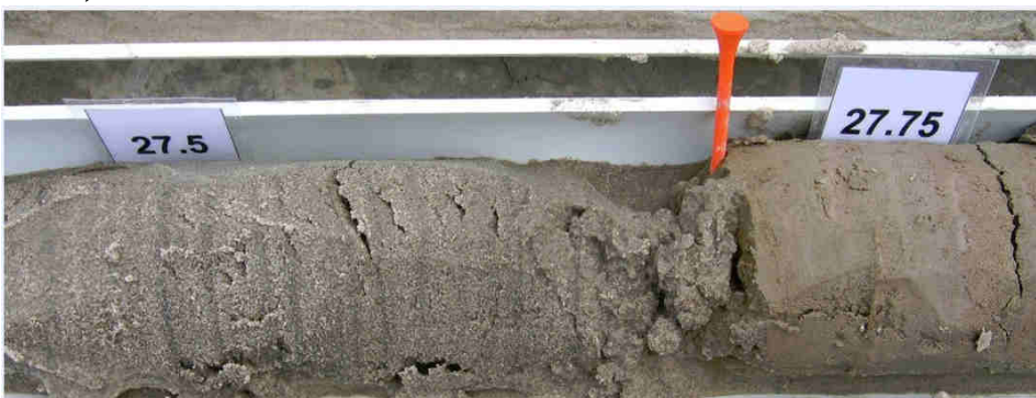
Photo 3: Example of Algonquin Aquifer unit with bedding planes. Marker indicates top of sequence of silty-clay laminations (OGS, 2006).
