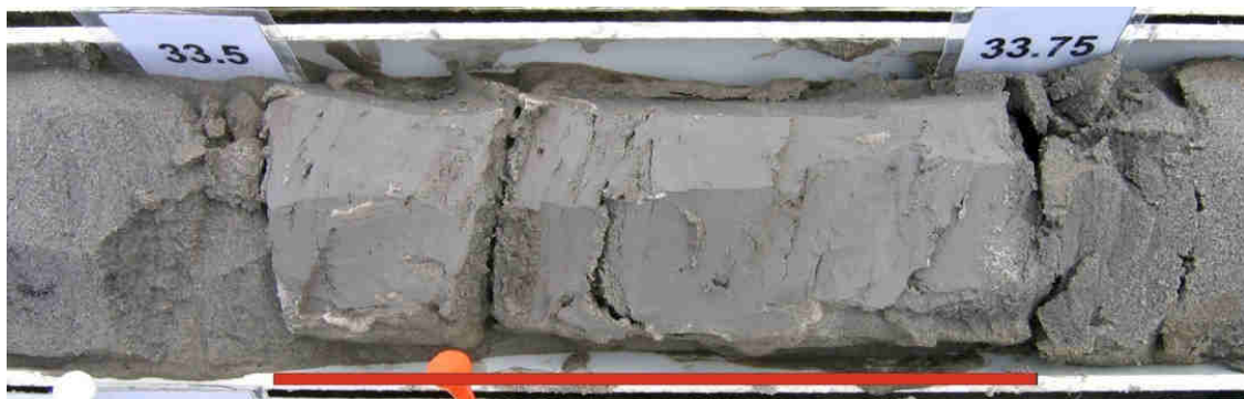
Photo 7: Example of transition into Algonquin Aquitard unit at 33.5 mbgs (OGS, 2006)
