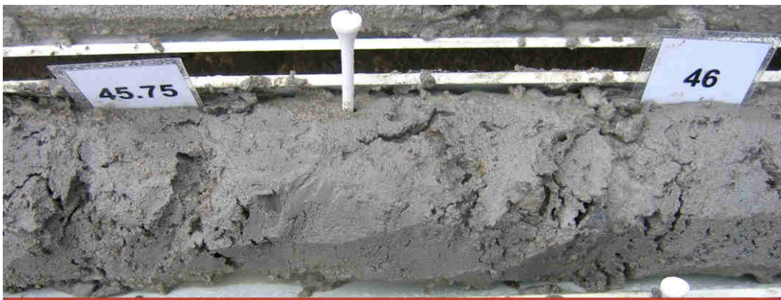
Photo 9: Example of sandy-silt diamicton bedding in the Upper Valley Filled Sediments Aquifer between 45.75 and 46 mbgs (OGS, 2006)
