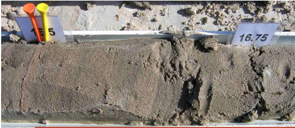
Photo 1: Example of Algonquin Aquifer unit with bedding planes. Markers indicate thin ( i.e. , 2-4 cm) sequence of silty-clay laminations (OGS, 2006).
