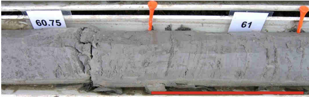
Photo 12: Example of the Middle Valley Filled Sediments Aquitard depicting rhythmically bedded silt and silty-clay between 60.75 and 61 mbgs (OGS, 2006).
