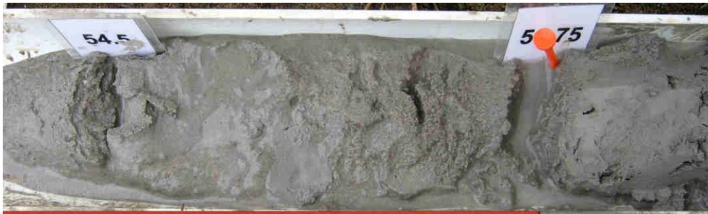
Photo 11: Example of Middle Valley Filled Sediments depicting medium textured saturated sands transition into sandy-silt diamicton at 55.75 mbgs (OGS, 2006)
