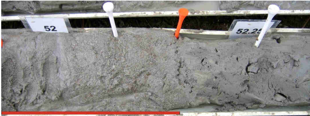
Photo 10: Example of sand (interbed) transition back in silty-sand diamicton in the Upper Valley Filled Sediments Aquitard (OGS, 2006).
