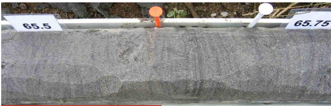
Photo 13: Example of lower aquifer sediments showing fine to medium bedded sand (OGS, 2006)
